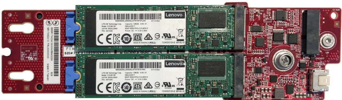
Figure 3. SATA/NVMe M.2 Module with 2 drives
