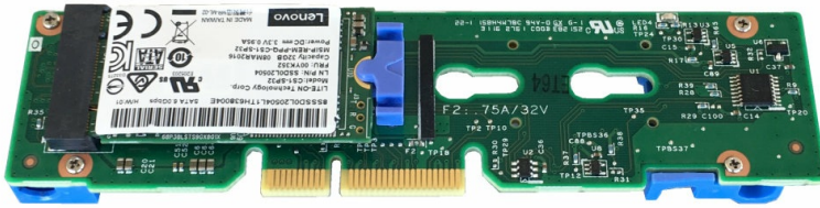
Figure 2. Single M.2 Adapter and a 32 GB M.2 drive
